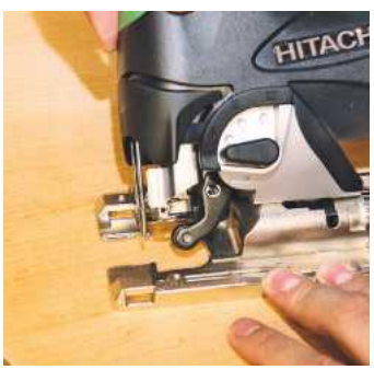
▲ Set at an angle the base sticks beyond the front of the saw...
